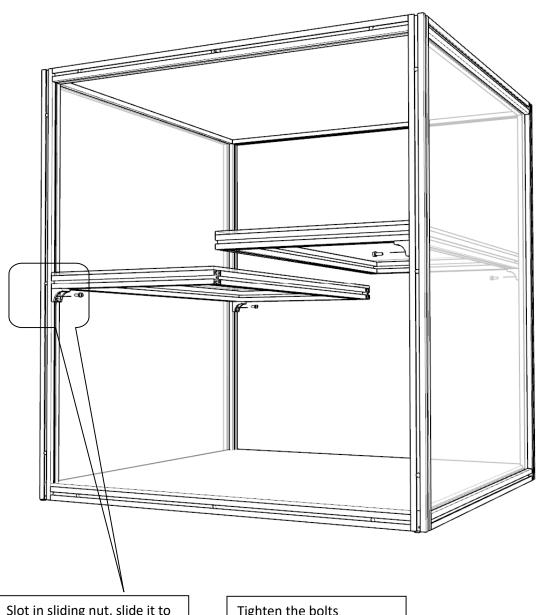
Slot in sliding nut, slide it to align with the angle bracket hole
