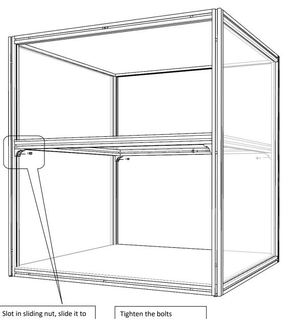
Slot in sliding nut, slide it to align with the angle bracket hole
