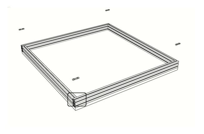
\*Slot in M4 nuts at an angle into the aluminium profiles
