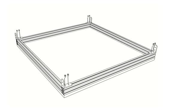
Insert shelf into display cube, secure with M4 bolts
