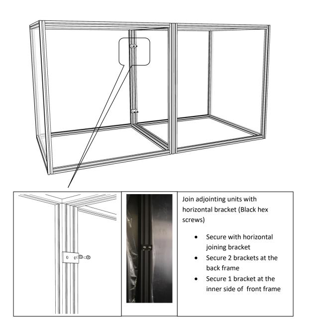
\*Note: Do not insert the side panels for the displays where the joints will be done
