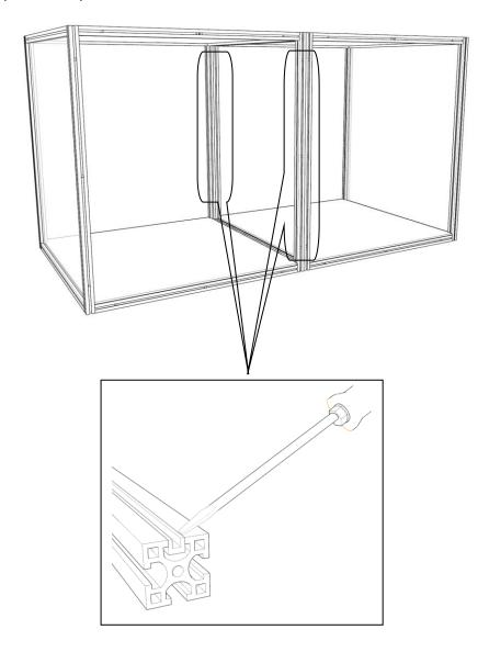
\*Note: Remove plastic holder with a flat head screw driver.
