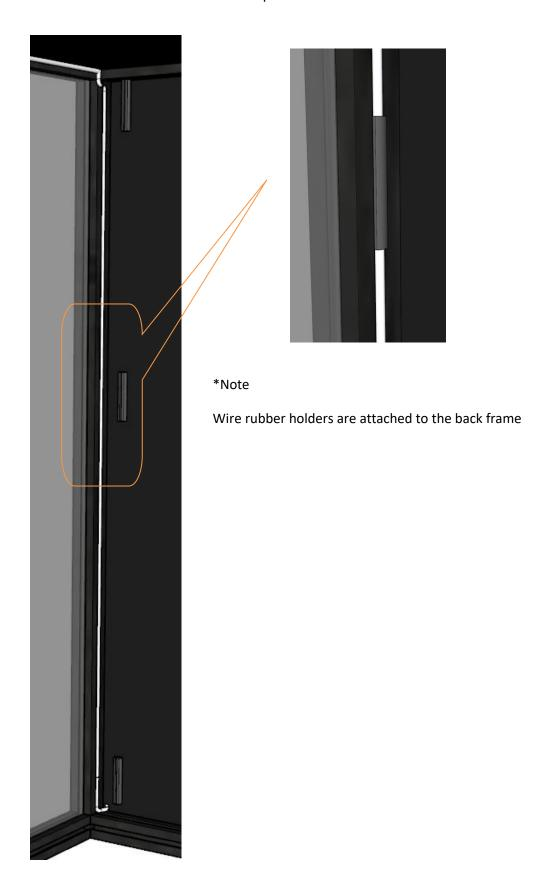
3c – Insert wires into the hole at the bottom left/right of the back panel
